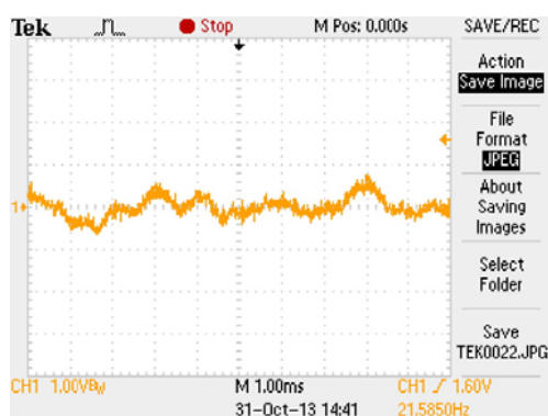
Vibration Wave form (700RPM, L=9.6m)
