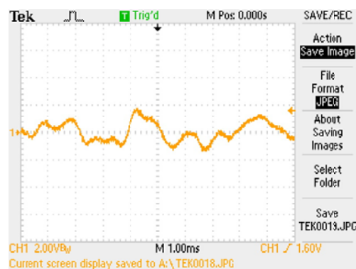
Vibration Wave form (700RPM, L=4.3m)
